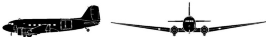
Fig. 1 DC-3 airplane. The requirements for the DC-3 included a payload of 21–32 passengers, a cruise speed of 200 knots and a range over 2,500 kilometres which was unprecedented at that time
