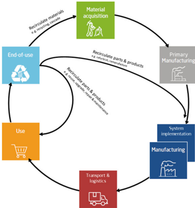
Fig. 4 A typical product or system life cycle (own figure)
