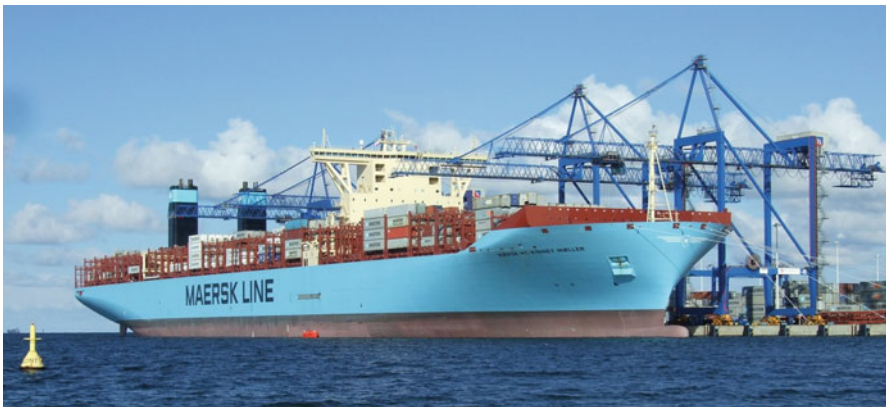
Fig. 12 The Mærsk Mc-Kinney Møller, one of the largest container ships in the world. It carries over 18,000 20-foot containers with a crew of 13. (Picture credit: Slawos 2013 – CC BY-SA 3.0)
