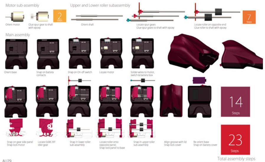
Fig. 11 Design for assembly analysis of a card shuffler after redesign. (Image from the author)
