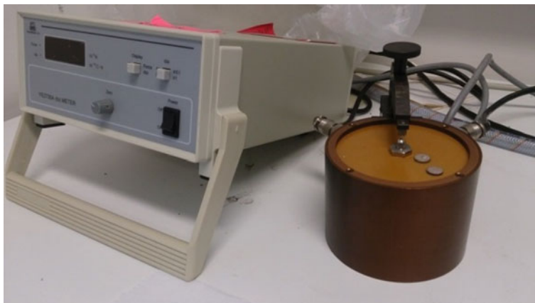
Fig. 2.13 D33 meter machine to measure piezoelectric constant of nanocomposite films
