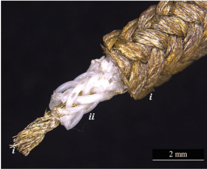
Fig. 3.2 Optical photograph of the as-developed triaxial braided piezo generator: (i) silver coated nylon as inner and outer electrodes and (ii) braided PVDF fibers as the intermediate layer. The structure had a total diameter of 2.55 mm consisting of a silver coated nylon core (0.6 mm), an intermediate PVDF layer with a thickness of 1.37 mm, and outer sheath of silver coated nylon braid with a thickness of 0.58 mm
