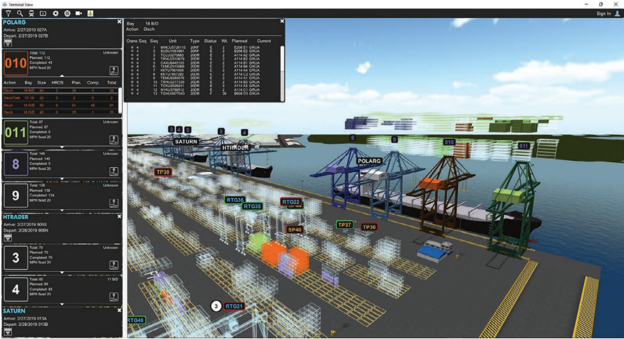
FIGURE 11.8 An interface of the 3D SPINNAKER application displaying the vessel operations filter functionality.
