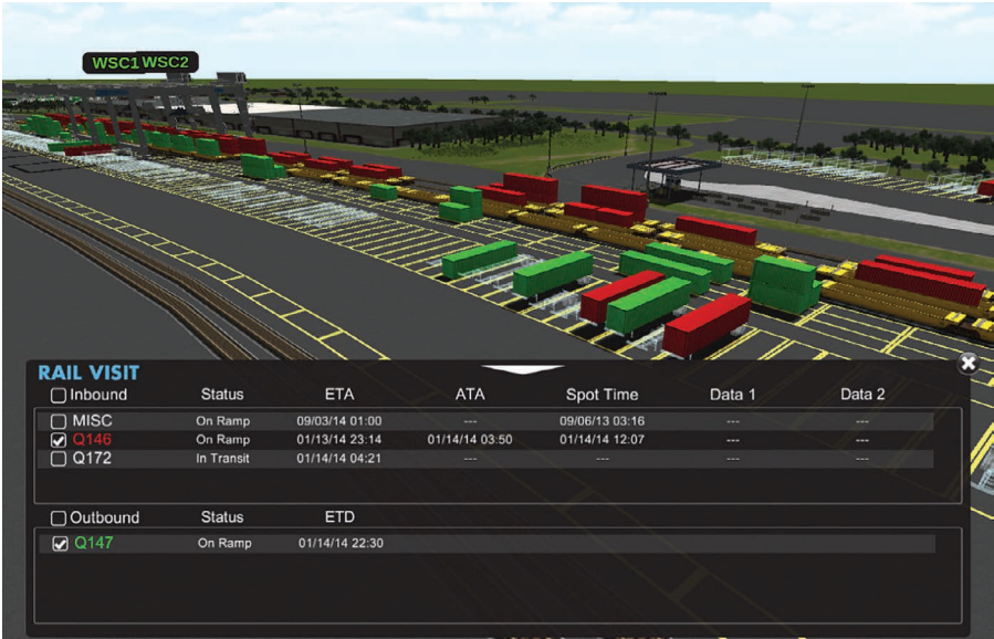
FIGURE 11.9 An interface of the 3D SPINNAKER application displaying the rail operations filter functionality.
