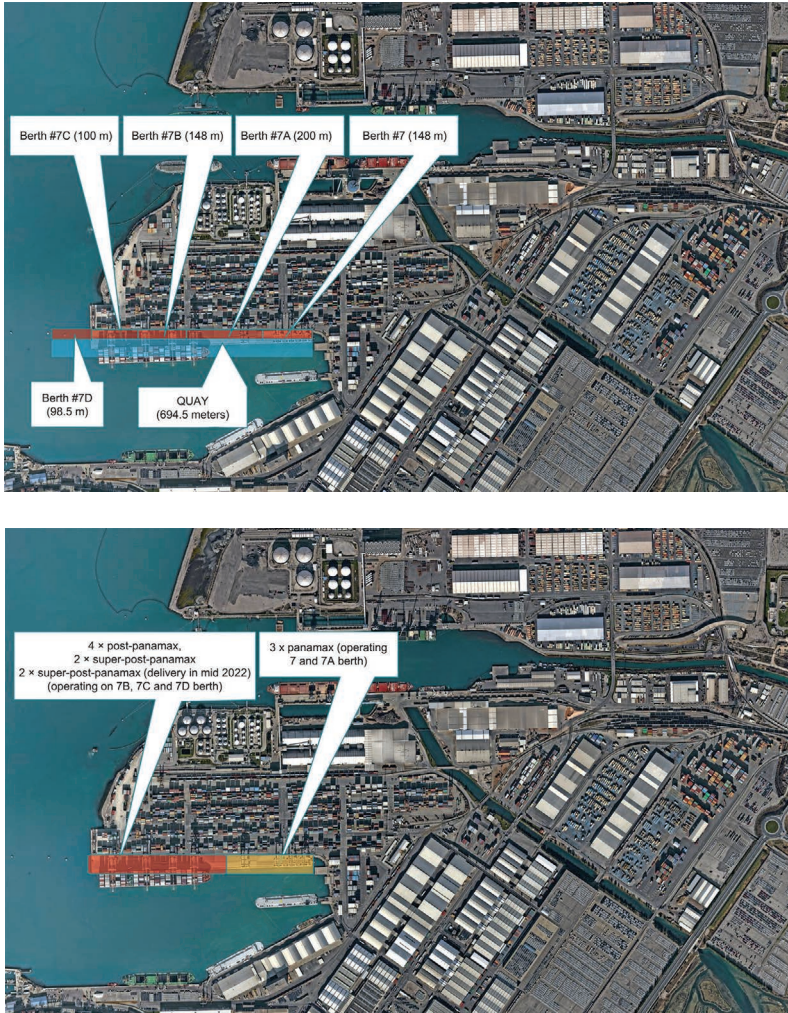
FIGURE 10.1 The wharf at the Luka Koper container terminal, including the operational range of the STS cranes.
