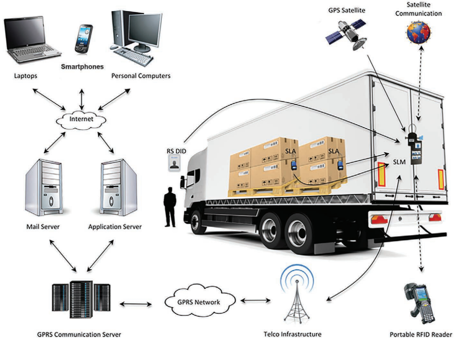
FIGURE 3.3 A scheme of transmitting information about events under the system of the RadioSecure electronic seal.
