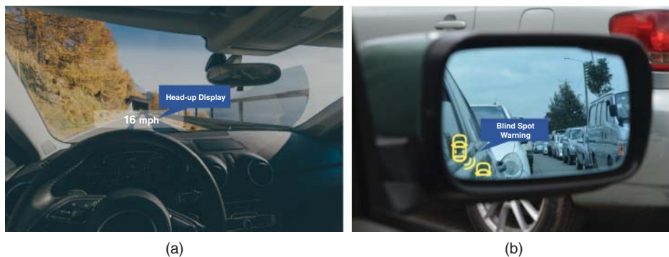
Figure 28.2 Heads up displays depicting (a) vehicle speed and (b) blindspot warning. Source: Riccardo/Pexels; Stan/Pexels.
