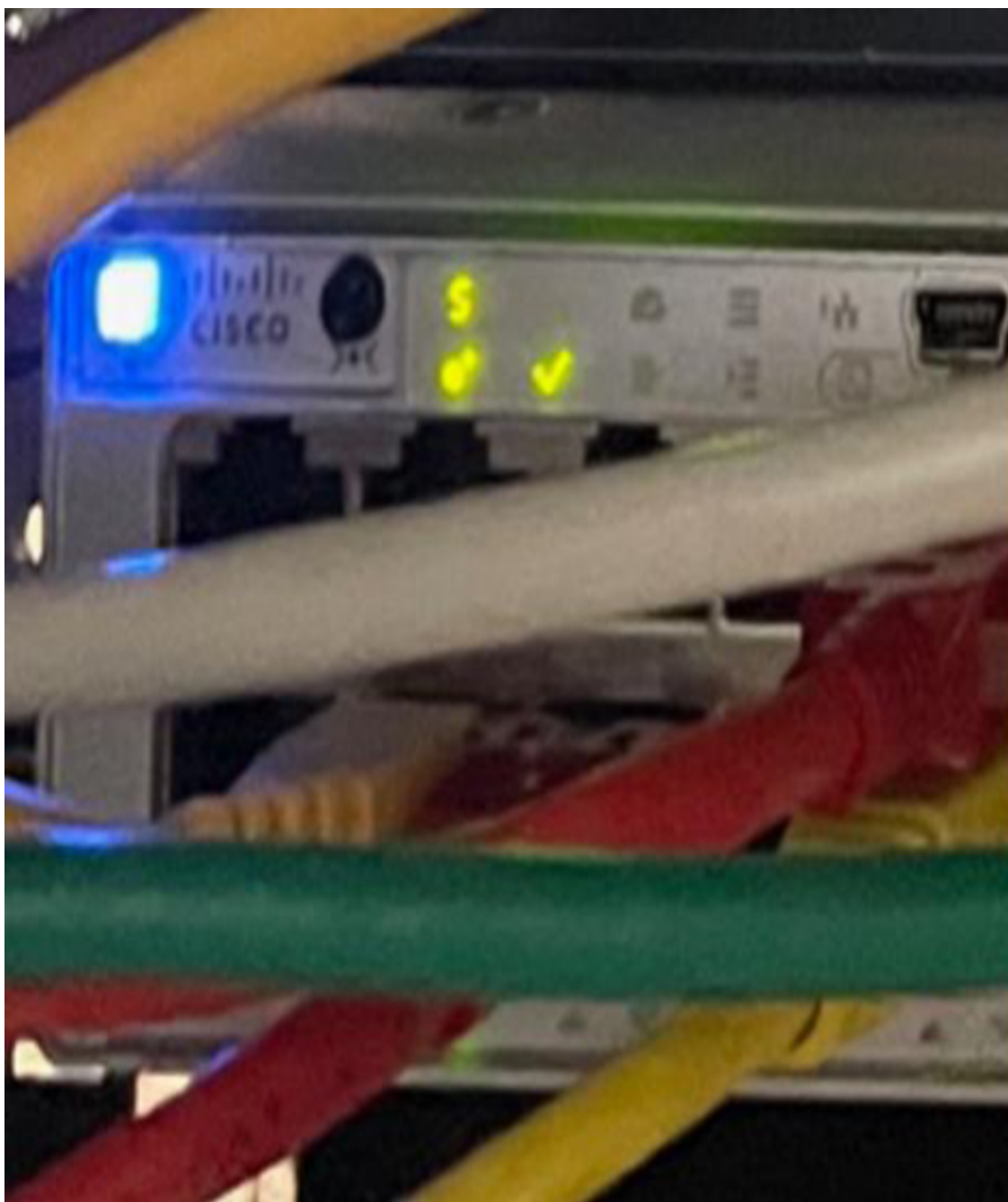
Figure 7-29 Blue Configurable Beacon on a Catalyst 9300 Series Switch
