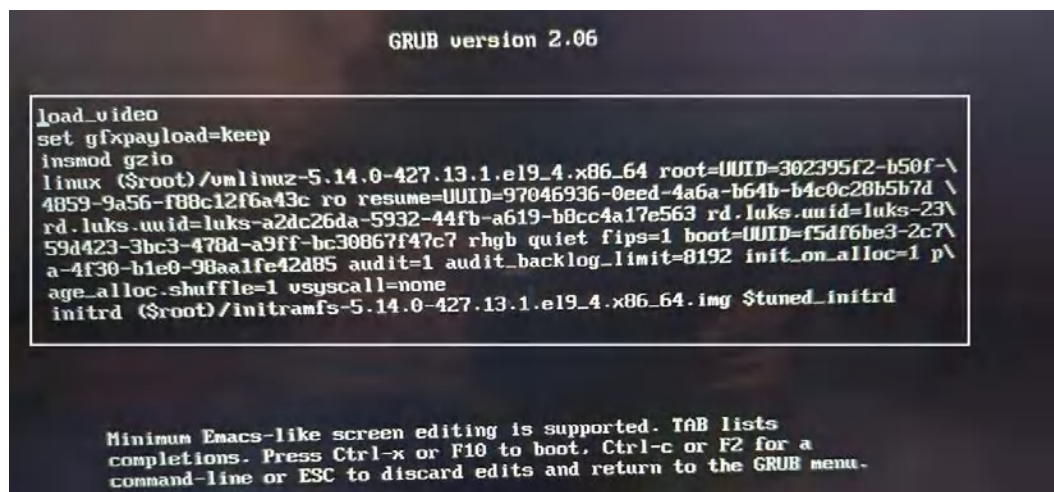
Figure 13.4 – Confirming FIPS mode boot options in GRUB
