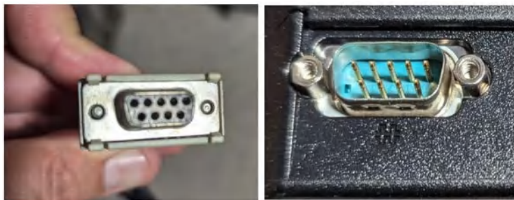
Figure 12.2 – Serial connector examples
