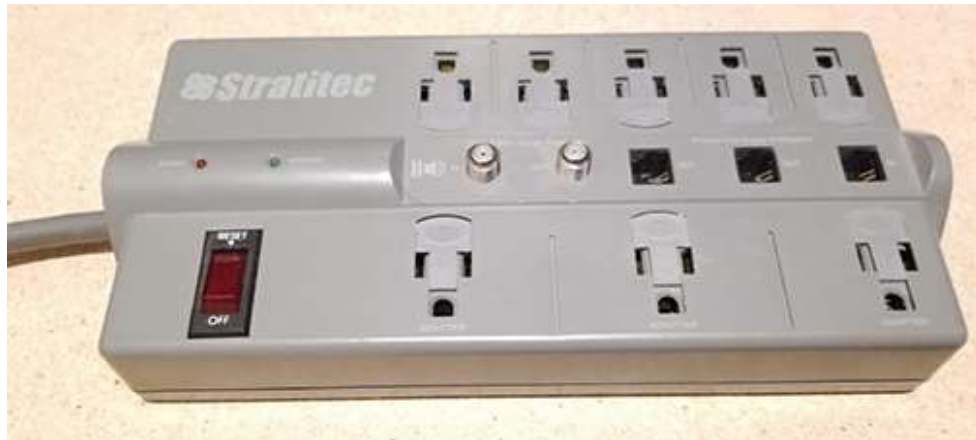
FIGURE 10.5 A common surge protector.
