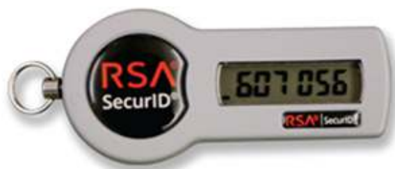
FIGURE 4.5 An RSA security key fob.
