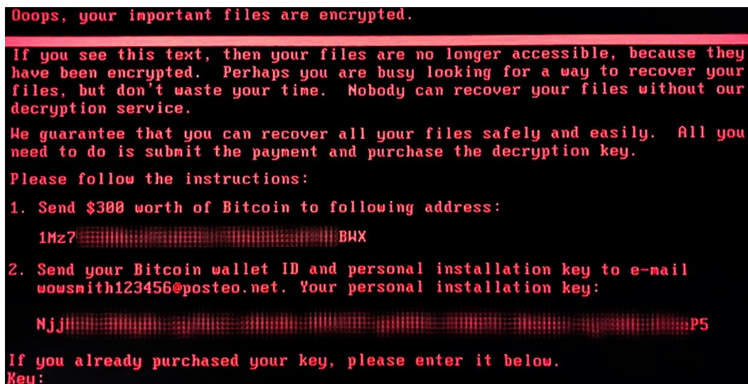
Figure 1.3 – The ID shown in the ransom screen is only plain random data (source: Securelist.com)
