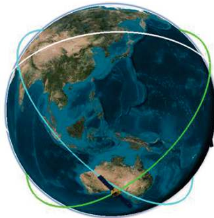
Figure 3.2 Delta constellation structure diagram (viewed from the pole).
