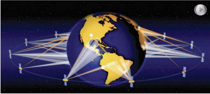
Figure 4.1. Medium earth orbit satellite constellation displaying customer and gateway spot beams.
