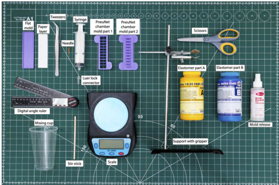
Figure 3.10: Preparation for laboratory example 3A: all of the materials required to make PneuNet actuators.
