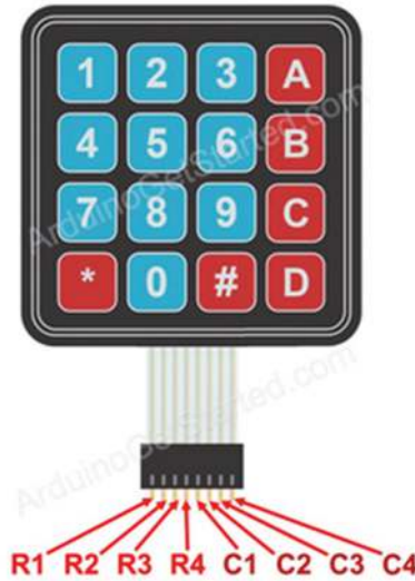
Figure 11.5 Pin configuration of the 4x4 keypad.
