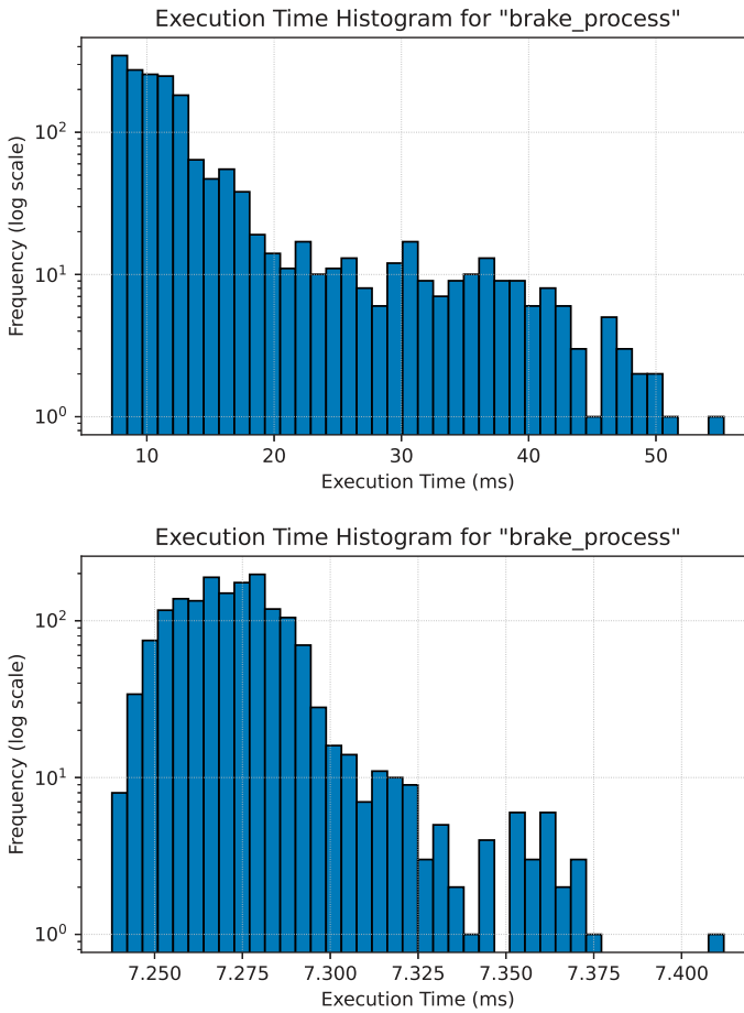
Figure 7.28: Execution time of the end-to-end processing of the critical path. Upper graph corresponds to non-real-time execution, and the bottom graph corresponds to real-time execution.
