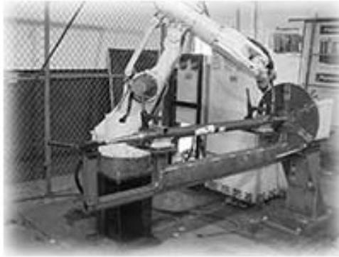
FIGURE 17.7 Robot Performing Sealing Operation.
