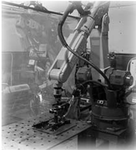
FIGURE 17.9 Robot Performing Drilling Operation.
