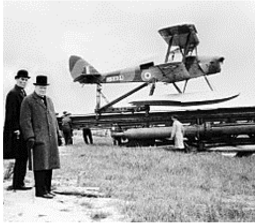
FIGURE 19.2 Launch of a DH.82 Queen Bee (mother of drones) target drone (1941) (Dronethusiast, 2020).
