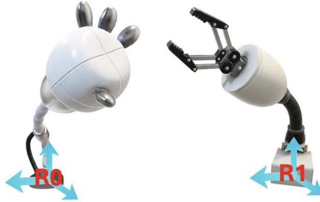
Fig. 2.25 Arm-type robots and the coordinate frames, where R_0 and R_1 are robotic coordinate frames on the bases
