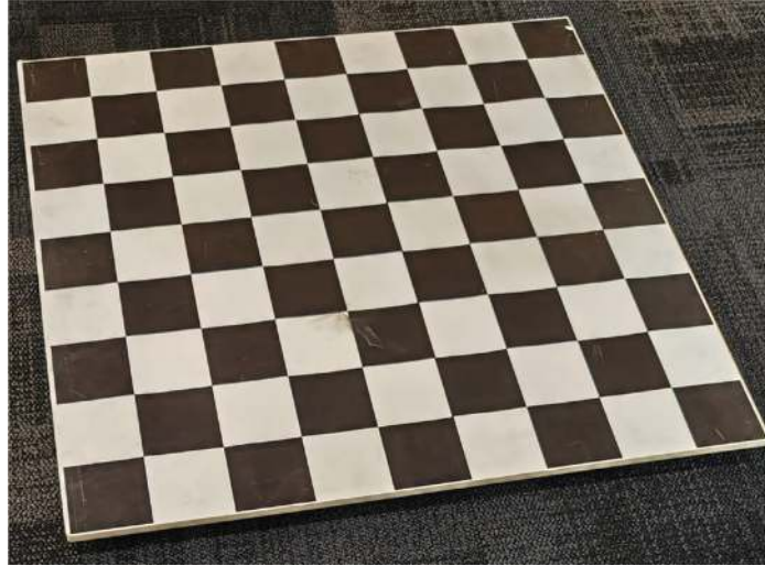
Fig. 3.4 Our chessboard for camera calibration
