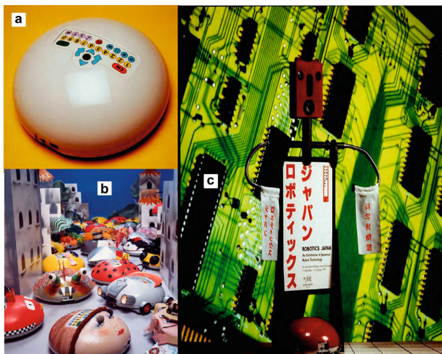
Fig. 3 a The Classic Roamer® a platform for constructionism. b Examples of children's designs. c Roamer® transformed into a greeting robot for the London Science Museum; it detected guests and told them how to get to the Japanese robot exhibition
