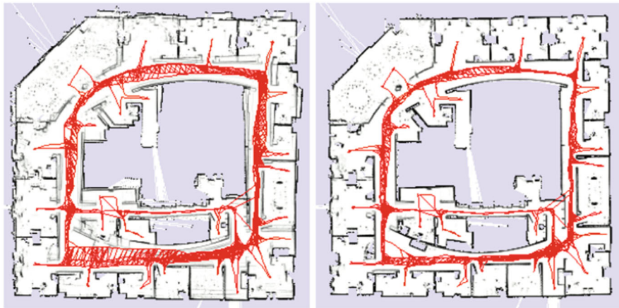
Fig. 10 Intel research lab. Left: unoptimized pose graph overlaid on top of the resulting map. Right: the optimized pose graph and the resulting consistent map
