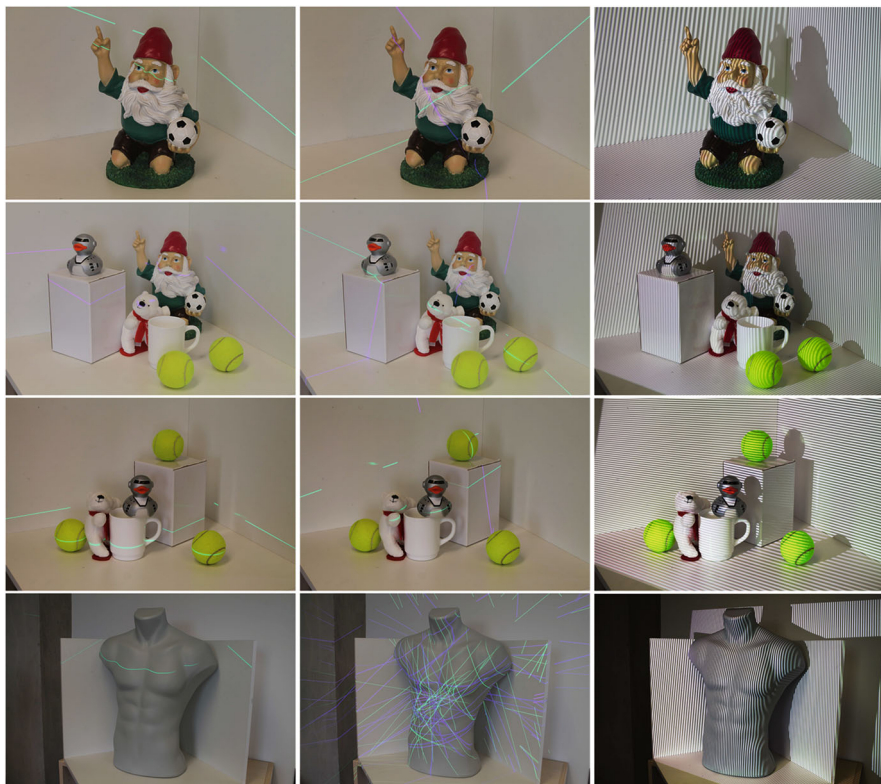
Fig. 15 Structured light in various scenes using a line projector (left), a cross-line projector (center) and a projected light pattern (right). Last row, center: the accumulated lines of 26 images. As the camera and the scene remain stable the intersection detection is performed with all images
