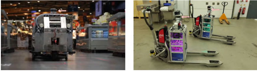
Fig. 3.6 Two types of service robots equipped with 3D lidar (pointed out by the red arrow)
