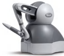
(b) The Geomagic Touch series of serial force feedback haptic devices [87]
