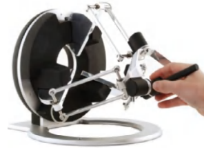
(c) The Omega series of parallel force feedback haptic devices by Force Dimension [87]
