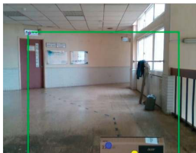
Figure 20. The robot finds an obstacle as the blue mark (in the middle area) and yellow mark (in the right area) on the picture, and the distances are 1.65 m and 1.62 m, respectively; the action is a LEFT turn.
