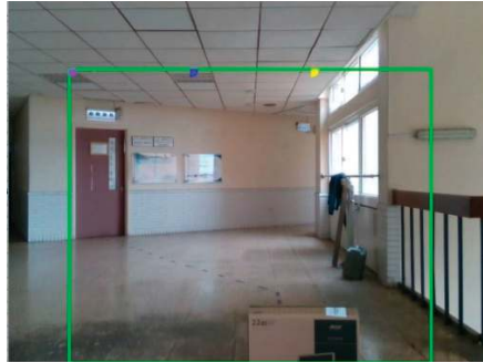
Figure 18. On the depth camera image, the distances of the nearest left, middle, and right objects are greater than 2 m, so the action is GO.
