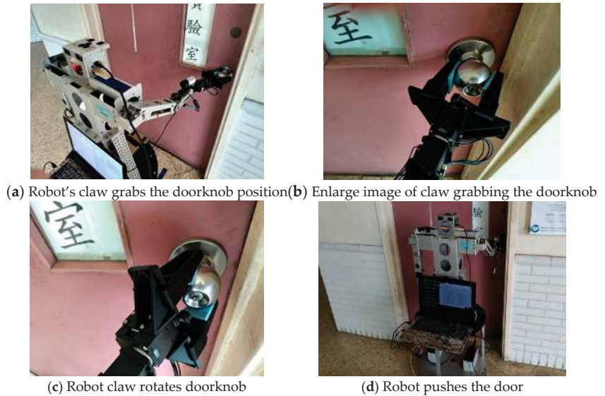
Figure 27. The robot opens the door; the Chinese characters on the figure are the room's name.
