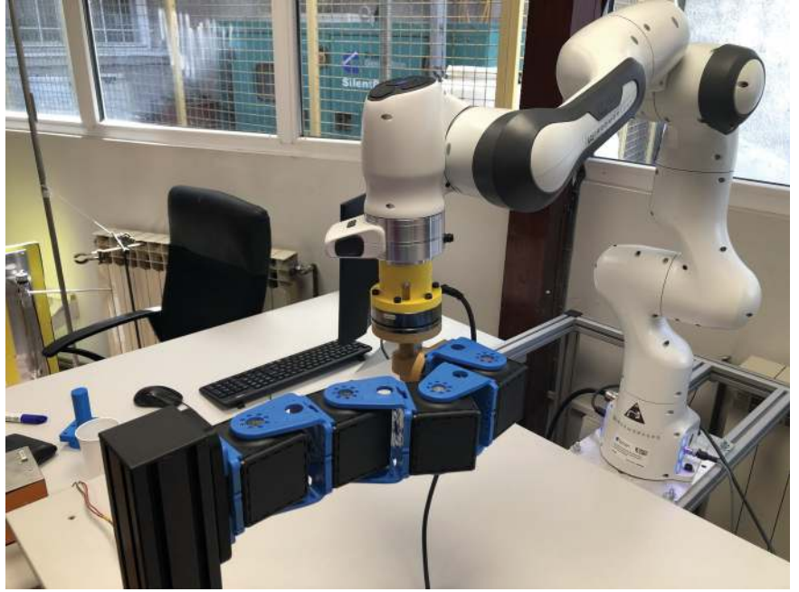
Figure 9. Experimental setup: 4 DoF planar robot with QB actuators, Franka Robotics Panda robot, and Axia80-M8 F/T sensor.
