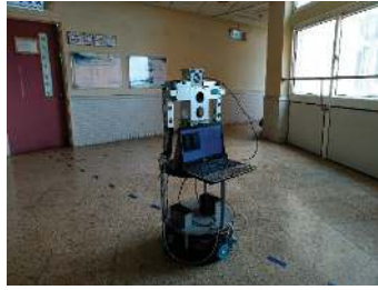
Figure 24. After the SURF matching, the robot turns to the target direction and moves forward.
