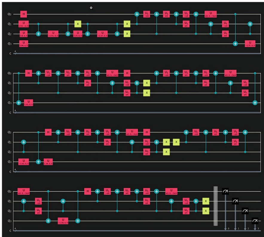
Fig. 14.7 Generated circuit from preparation code
