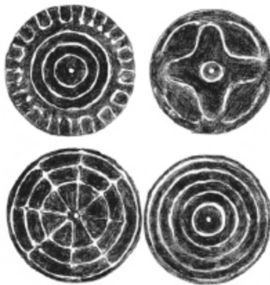
Chladni patterns: the white lines are the places where the rice gathers (the nodes). Here, the wave doesn't move.
