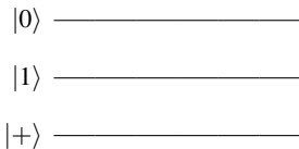
Figure 2.4 The structure of a quantum circuit. Qubits are initialized, and computation flows from left to right. This circuit has no gates yet.
