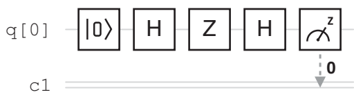
Figure 2.3. Deutsch’s algorithm with a phase oracle for a balanced function, created using IBM Quantum.
