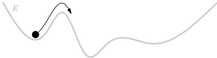
Fig. 7.1 Caricature of the energy function and macro state of a Hopfield net. In the situation shown, the state of the network is trapped in a local minimum of the energy function. Asynchronous updates of individual neurons will only take effect if they decrease the energy and even then would only locally move the macro state. Under asynchronous local updates, the current state is therefore stable and cannot escape from its position. This would instead require (several) steps in a direction of increasing energy after which the network could proceed towards the global minimum of its energy function
