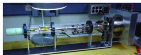
Insert for  $^4\text{He}$  cryostat
