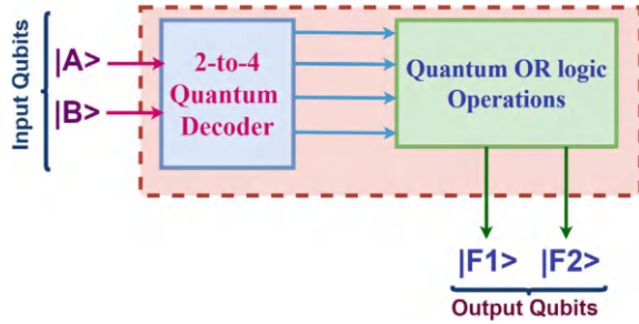
Fig. 2.7 Block diagram of quantum 4-to-2 ROM
