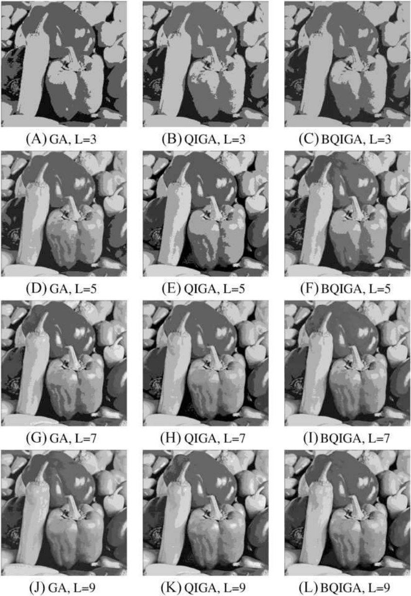
Figure 8.4 Segmentation output of Sample-2 for different levels and algorithms. BQIGA , Bi-level quantum-inspired genetic algorithm; GA , genetic algorithm; L , gray level; QIGA , quantum-inspired genetic algorithm.
