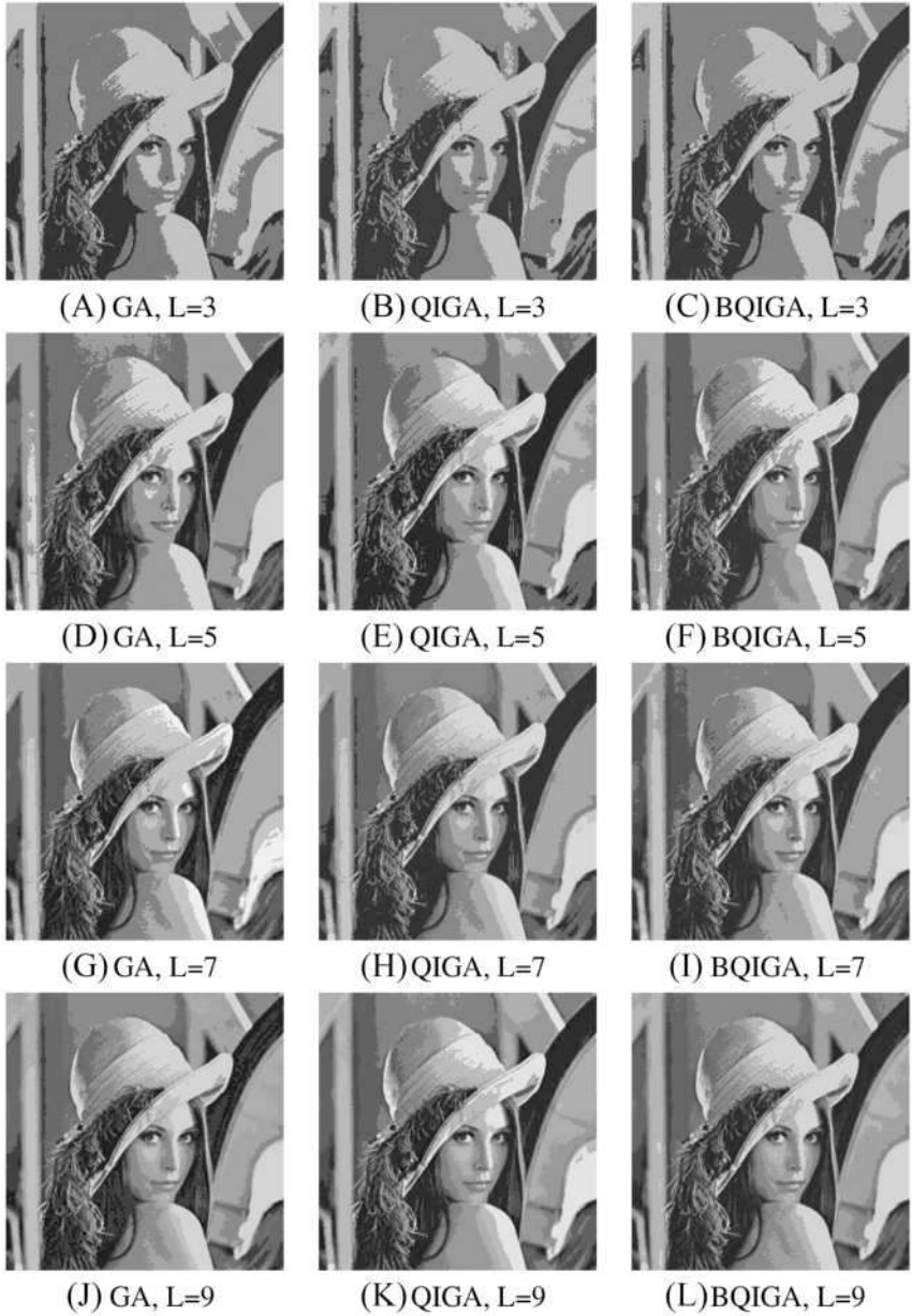
Figure 8.3 Segmentation output of Sample-1 for different levels and algorithms. BQIGA , Bi-level quantum-inspired genetic algorithm; GA , genetic algorithm; L , gray level; QIGA , quantum-inspired genetic algorithm.
