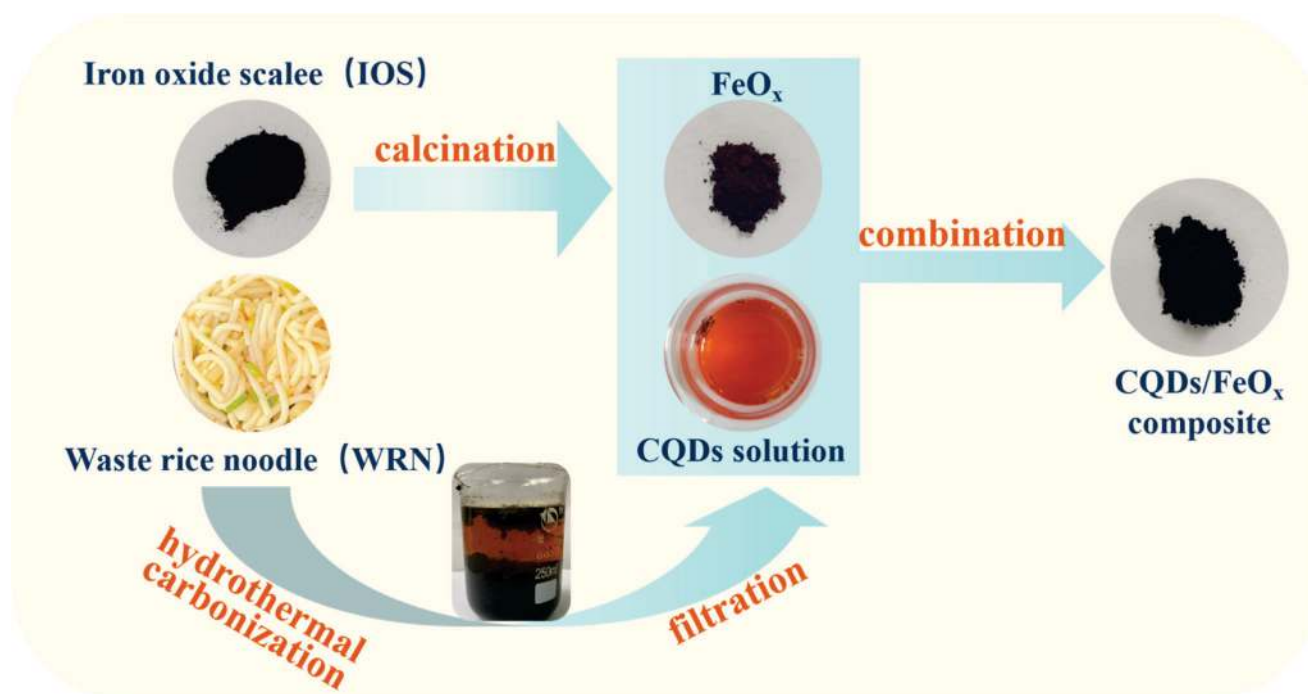
Figure 1. Formation process of CQDs/ \text{FeO}_x composite using WRN and IOS as raw materials.
