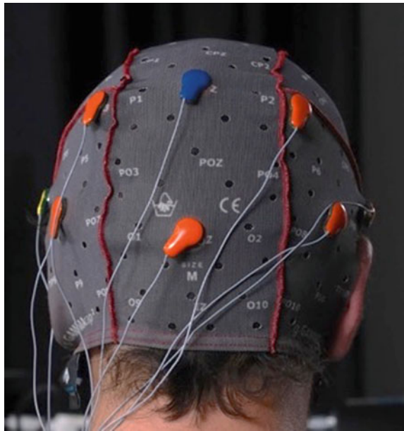
Fig. 2 Cap furnished with electrodes relay EEG data to a computer for further processing
