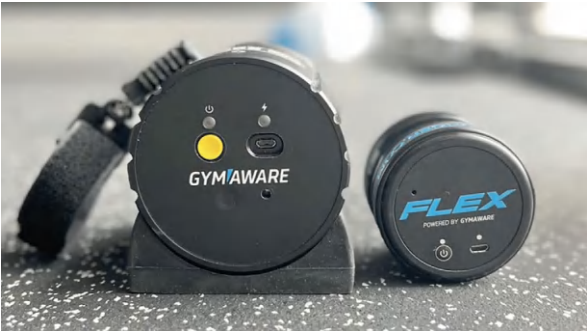
Fig. 10.2 GymAware accelerometer. The GymAware accelerometer is an example of a sensor system used for velocity goal-based training
