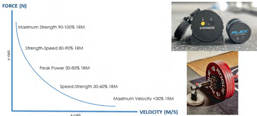
Fig. 6.5 Training zone force-velocity curve and examples of barbell velocity sensors
