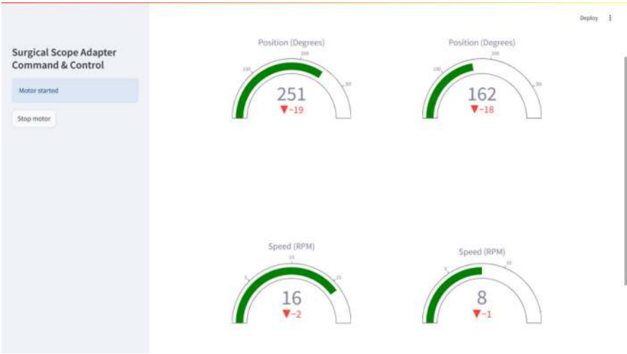
Figure 14-8. Streamlit command & control dashboard for the surgical scope adapter
