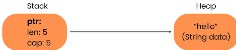
Figure 4.3: A String’s memory layout: stack-allocated metadata ( ptr , len , cap ) pointing to its heap-allocated data
