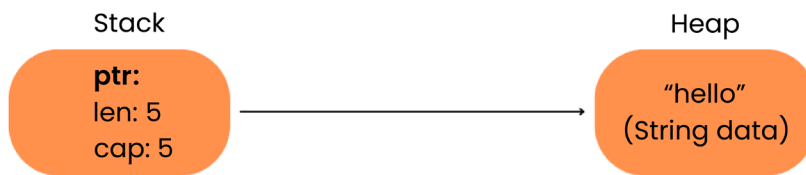
Figure 4.1: A String variable s1 on the stack, pointing to its heap-allocated data
