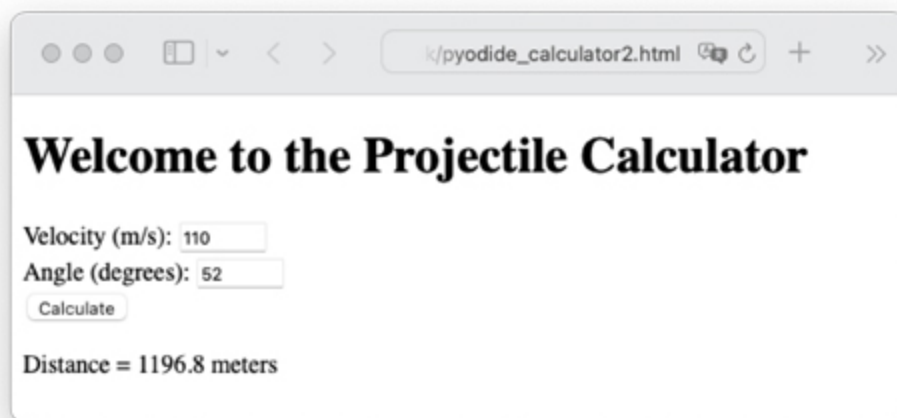
Figure 4.6 Projectile Calculator Web Application with Pyodide
