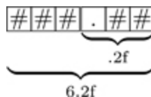
Figure 1.1 Example Fixed Point Number Spacing for Width = 6, Precision = 2
