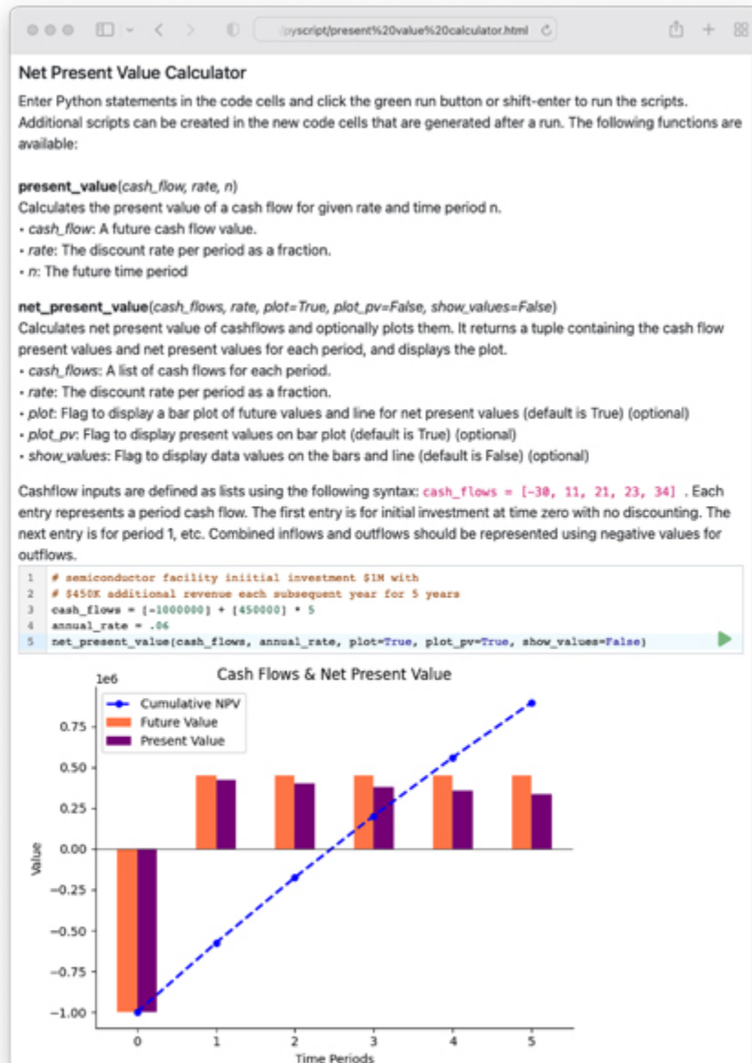
Figure 4.8 Present Value Calculator with PyScript and Matplotlib
