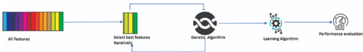
Figure 9.3: The process of feature selection using GA
