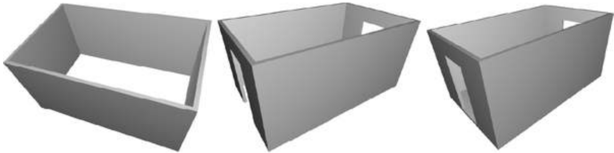
Figure 10-23. Adding the ground: using Boolean operations
