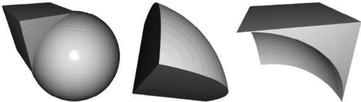
Figure 10-22. An example of CSG using the subtraction operation to create a complex shape from simpler primitives
