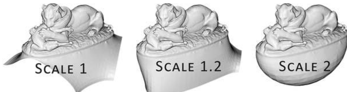
Figure 10-8. Impact of Poisson reconstruction parameters
