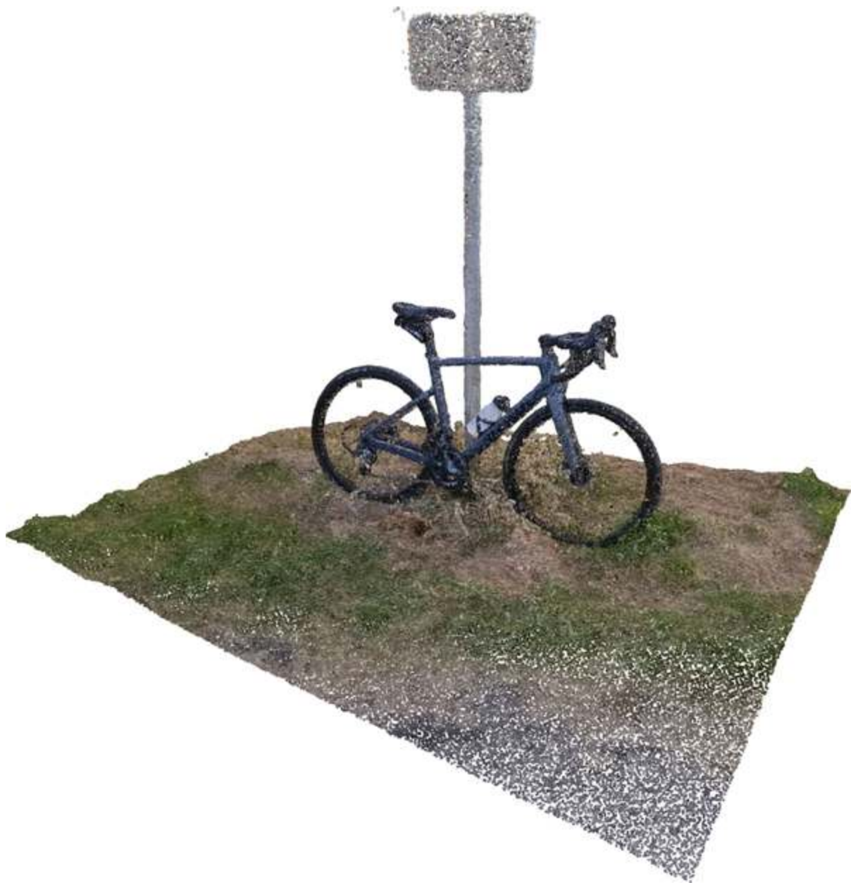
Figure 4-5. A 3D point cloud of a bike, with RGB color information
