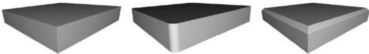
Figure 10-21. Fillet and chamfer example
