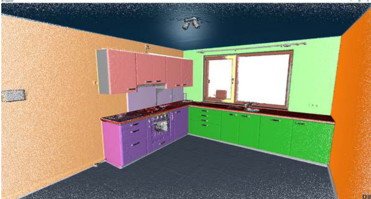
Figure 12-31. Downhill skiing approach in RANSAC: refining segments with iterative clustering and point selection
