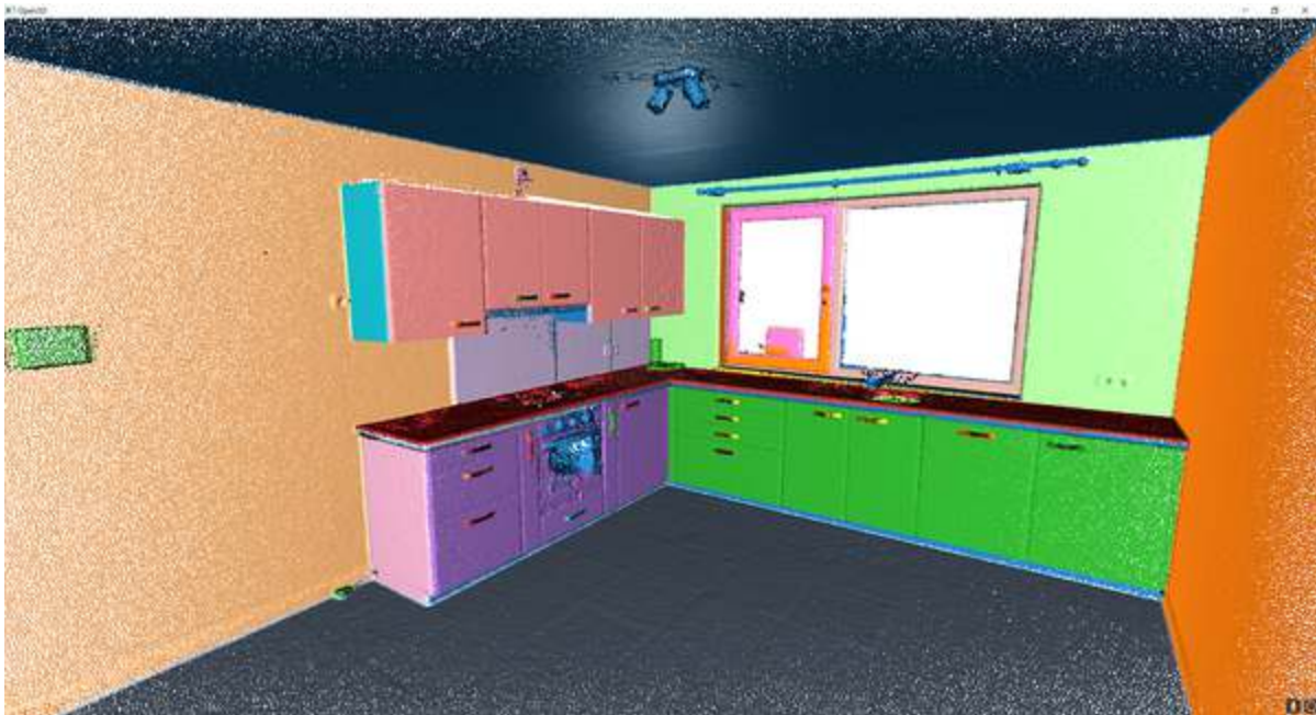
Figure 12-32. Final clustering outcome: applying DBSCAN to remaining points for complete point cloud segmentation
