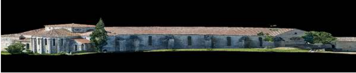
Figure 4-8. Example of a widely deformed cylindrical projection of the point cloud
