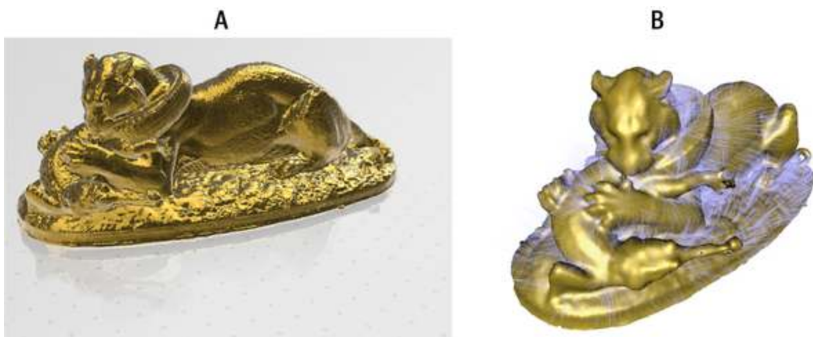
Figure 10-10. (A) This is a possible “gold print” of our 3D mesh, which is 20 cm long; (B) The visualization of the normals on the 3D mesh
