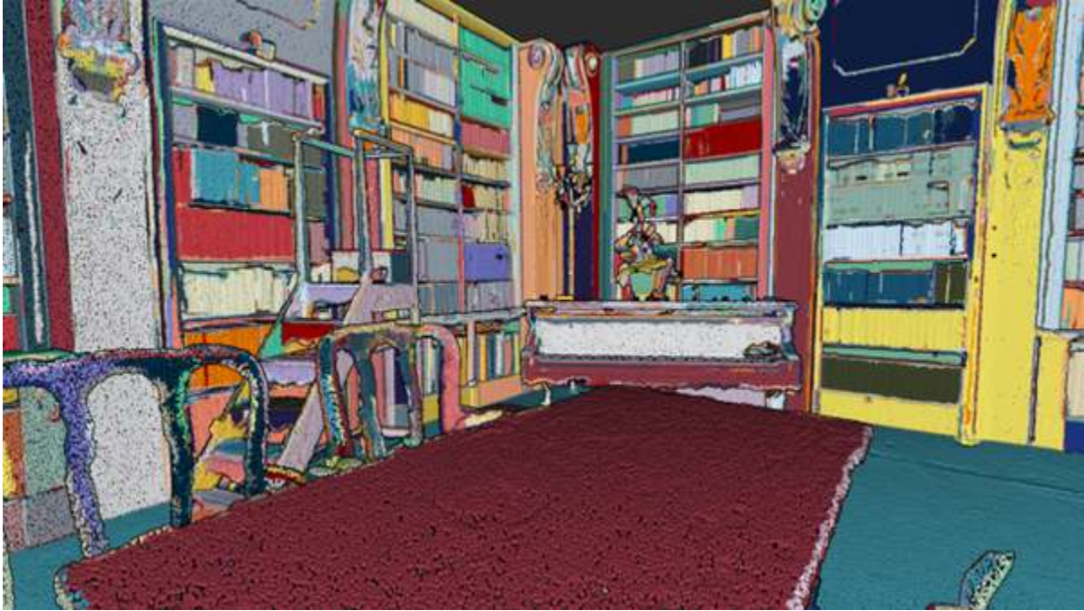
Figure 1-18. Example of a decomposition of a 3D point cloud dataset of a library into its main constituents
