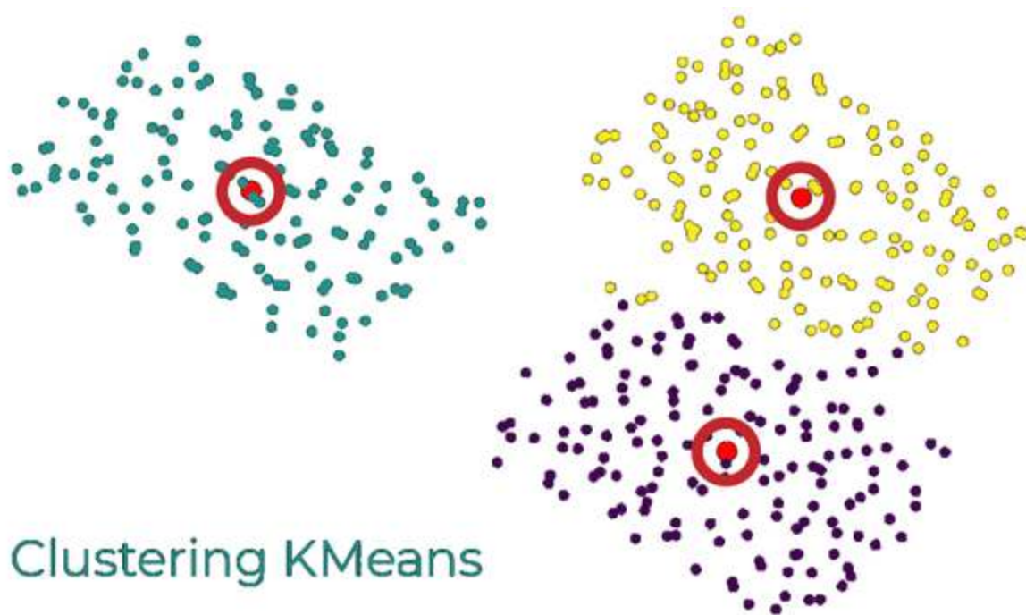
Figure 12-15. k-means clustering, showing how data points are assigned to clusters based on their proximity to cluster centroids
