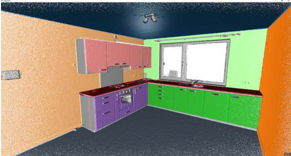
Figure 12-30. The outcome of the iterative RANSAC point cloud segmentation process
