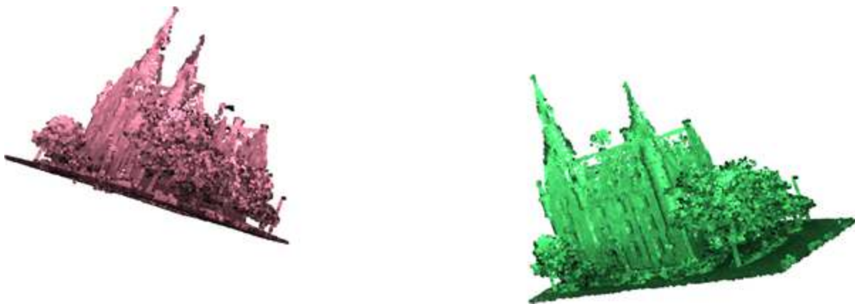
Figure 6-19. Fine registration using iterative closest point
