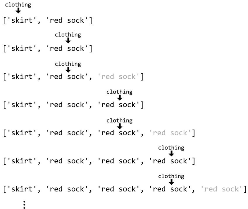
Figure 8-1: On each iteration of the for loop, a new 'red sock' is appended to the list, which clothing refers to on the next iteration. This cycle repeats forever.
