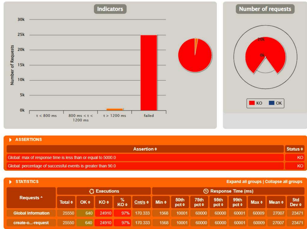
Figure 10.9 – Enabling virtual threads revealed a bottleneck in the database connection pool
