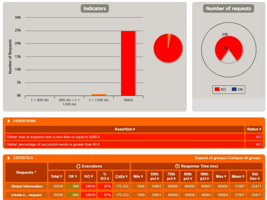
Figure 10.8 – Most of the requests failed as the service was not able to cope with the load
