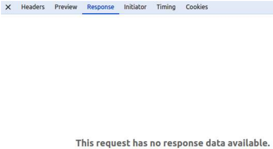
Figure 10.5 – No content is returned with the “304 Not Modified” response
