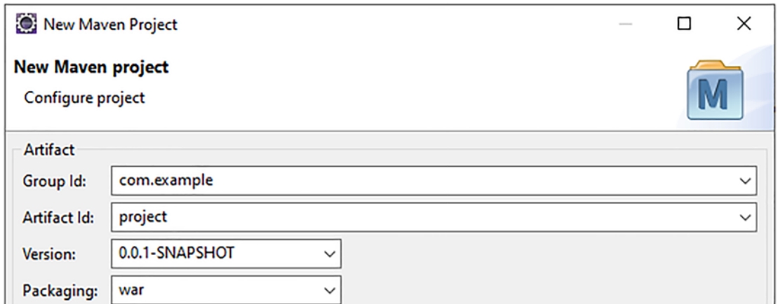
Figure 2-10. Filling out the Maven GAV in New Maven Project wizard
