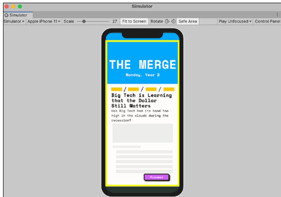
FIGURE 10-7: The device simulator is a useful tool for testing across mobile devices.
