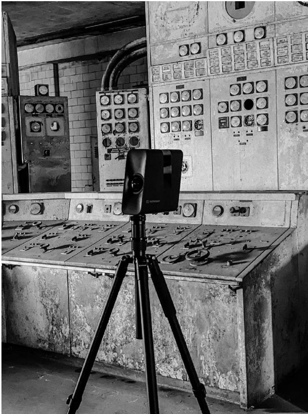
Figure 3.5.8 Terrestrial LiDAR Scanner in Control Room. Hearn Generating Station. Zak Fish.
