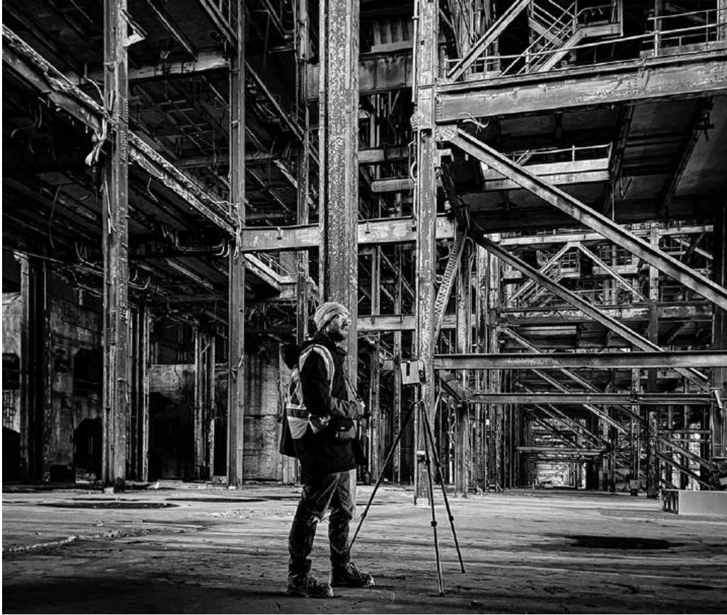
Figure 3.5.9 Technician operating Terrestrial LiDAR Scanner in Boiler Hall. Hearn Generating Station. Zak Fish.
