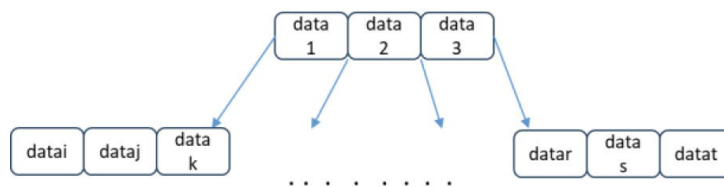
Figure 2-21 Modeling of multi-key search trees in C structures
