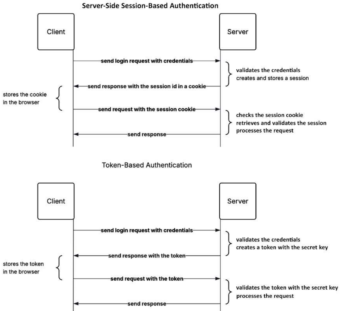
Figure 2.2: Server-side session-based authentication versus token-based authentication
