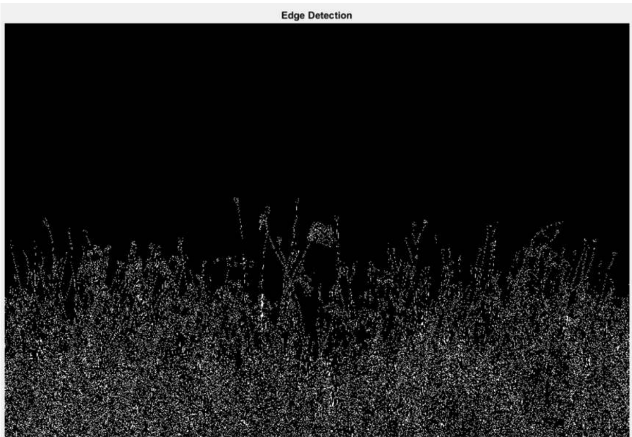
Figure 11.3: Edge detection using the Canny method in MATLAB
