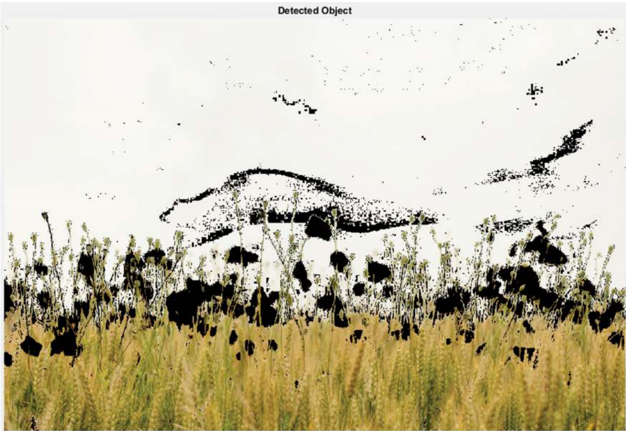
Figure 11.39: Object detection using color thresholding in MATLAB
