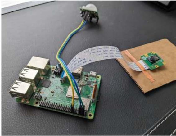
GPIO pin 18 that we attached to the PIR signal (SIG) lead. Whenever a hand or a bird wing waves near the PIR sensor, we should see a signal sent to the Pi's GPIO pin that we're monitoring.
