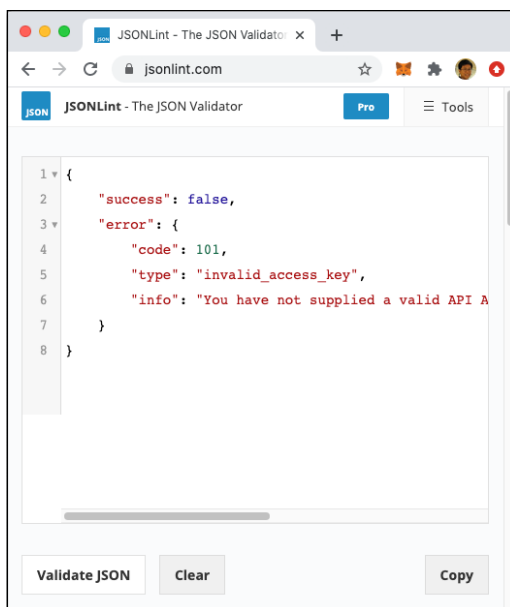
FIGURE 15-4: Examining the structure of the JSON error result returned by the Fixer API.
