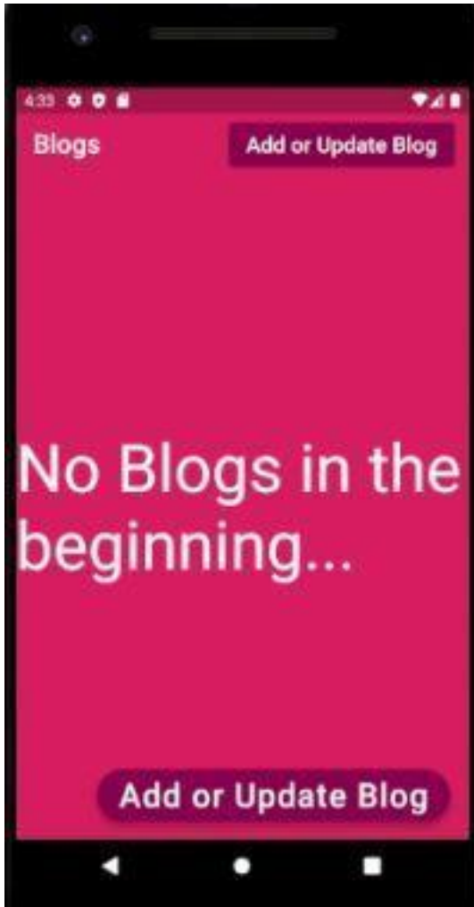
Figure 8.13 – Adding a Floating action button to SQLite Blog Home page in Flutter
