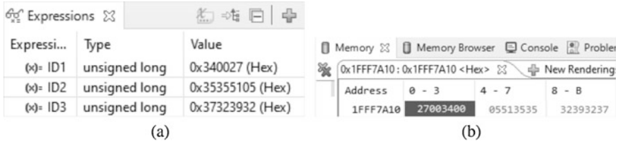
Fig. 9.5 Obtaining unique ID of the STM32F4 microcontroller. (a) Expressions window. (b) Memory map
