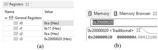
Fig. 15.2 Output of the second assembly code. (a) “Registers” window. (b) “Memory Browser” window
