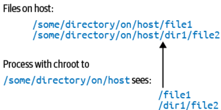
Figure 3-1. Changing root so a process only sees a subset of the filesystem
