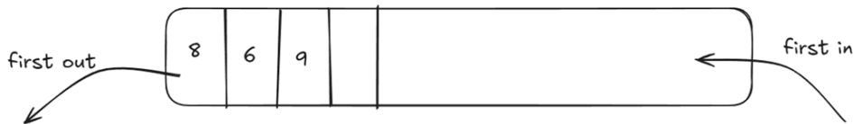
Figure 1.7 The queue data structure is First In First Out(FIFO). The number 8 illustrated in the image was inserted first, and it will be popped out first.
