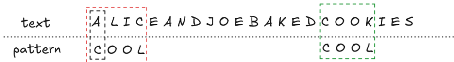
Figure 4.1 The pattern COOL is to be matched with the text "ALICEANDJOEBAKEDCOOKIES" . Each character is checked one by one. The first box shows that A and C are compared. With no successful match, we move the pattern forward by one character and continue comparing. The second box shows three characters matched, and the last character doesn't, concluding the pattern is not in the text only after checking the first three characters.
